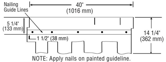
Figure 15-6: Fastening Presidential and Presidential TL Shake shingles on low and standard slopes.
