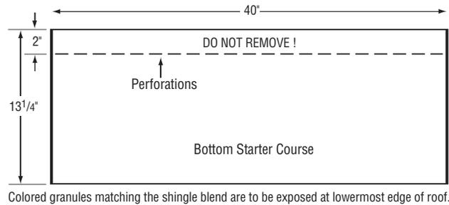
Colored granules matching the shingle blend are to be exposed at lowermost edge of roof.
